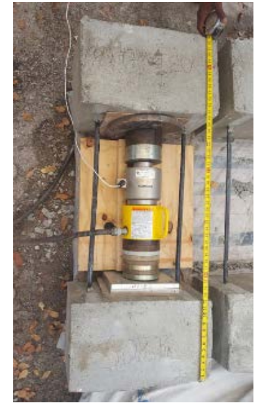
ASTM D7914 Strength of Bars at Bends
